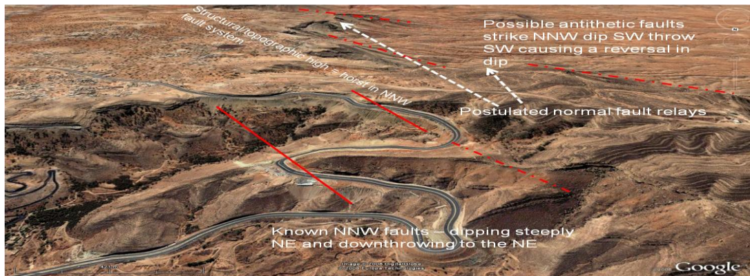
Fig 4. Nafusah escarpment north of the village of Abu Ghaylan. Kiklah Formation displaced by two major normal faults of the Jabel Nafusah system and forming a broad, low amplitude anticline between them.
